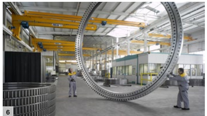
6 Completed large diameter bearing
