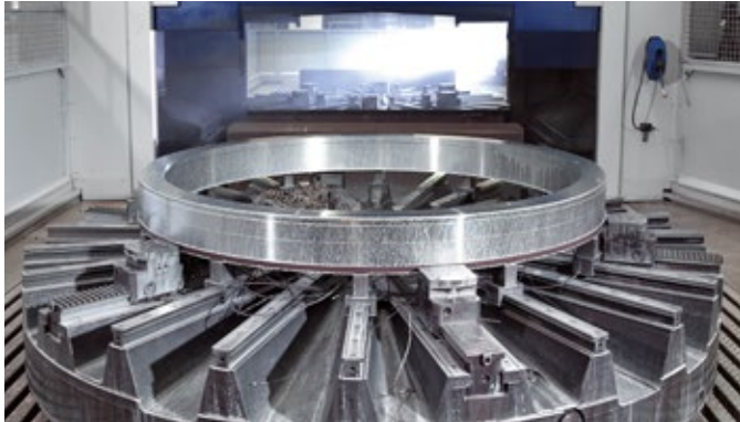
Manufacturing process - Turning
