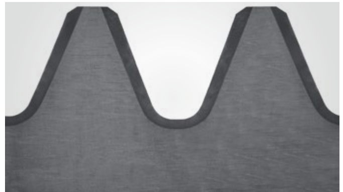
Hardening microsection of tooth spacing hardening
