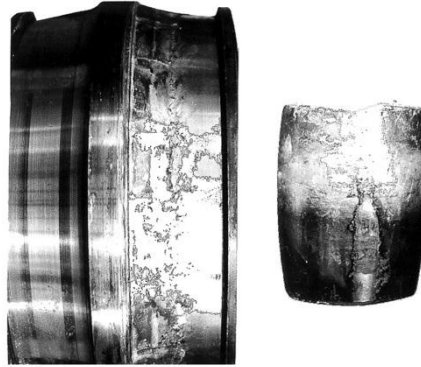
Fig. 4 – Discolored and melted running surfaces due to rolled wear particles from steel cage
